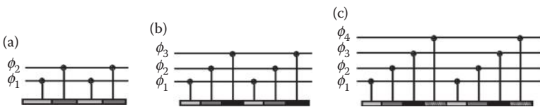
FIGURE 14.60 Two, three and four phase CCDs. (a) Two phase (b) three phase and (c) four phase.
